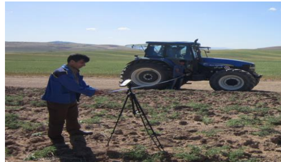
Fig. 2. How to measure the noise of the tractor in the surroundings positions.
