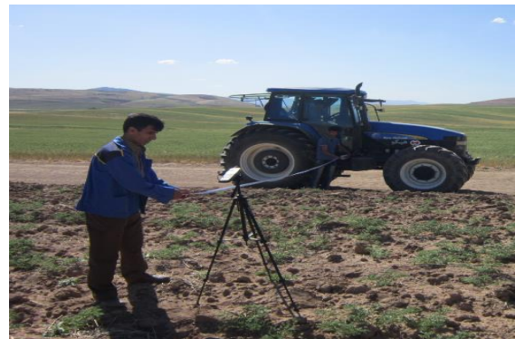
Fig. 2. How to measure the noise of the tractor in the surroundings positions.
