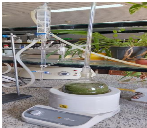
Fig. 1. Extracting essential oils from the Froriepia subpinnata plant using a Clevenger apparatus.
