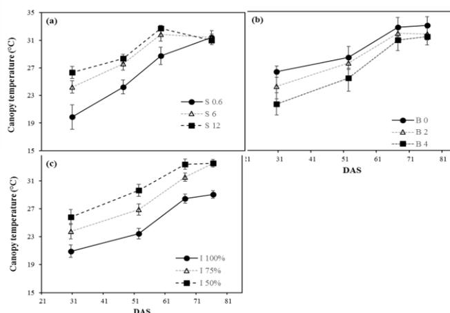
**Fig. 3.** Green canopy temperature (°C) at different irrigation, salinity, and biochar levels. Bars indicate the standard error of the mean.
