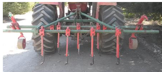
Fig. 4. The bent leg tillage implement
