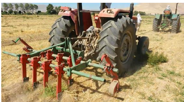
Fig. 5. Measuring draft force with a drawbar dynamometer and two tractors method
