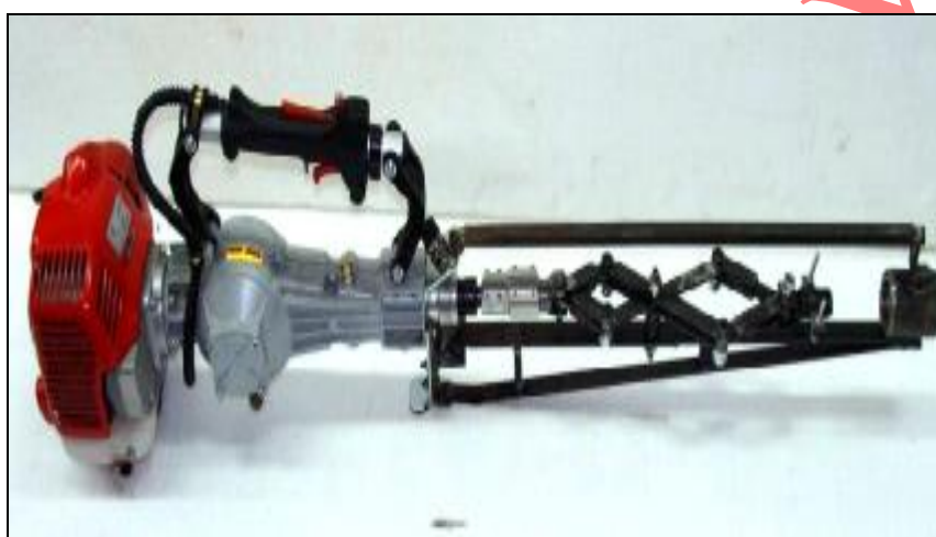
Fig. 1. The hand-held shaker and the the amplitude changing mechanism used for shake harvesting trials. (Shaker boom and hook not shown)
