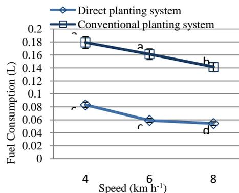
**Fig. 4.** Effect of cropping systems and speed on the average fuel consumption
