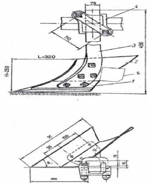
Fig. 2. Jointer: 1- share; 2- moldboard; 3- shank; 4- yoke; 5- drill seed tube holder (all measuring in mm).
