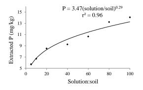
**Fig. 1.** Effect of NaHCO<sub>3</sub> solution: soil ratios on P extracted for 12 calcareous soils.
