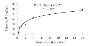
**Fig. 2.** Effect of shaking period on the P extracted by NaHCO<sub>3</sub> solution for 12 calcareous soils.
