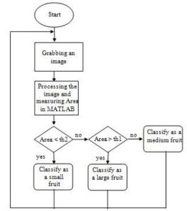
Fig. 5. Comprehensive sorting algorithm based on area
