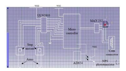
Fig. 3. Layout of the control circuit
