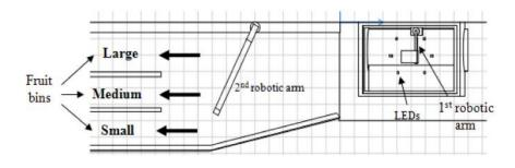
Fig. 2. Top view of the sorting rig
