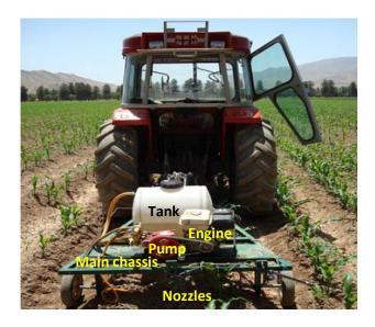
Fig. 1. The prototype site-specific herbicide application system developed in this study
