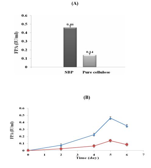
Fig 1. Cellulase production by *T. reesei* using SBP and pure crystalline cellulose as substrates.
