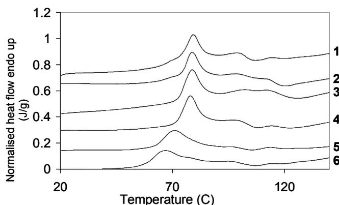
Fig. 1. DSC traces of the starch component of different rice powders determined by DSC. 1: Neda, 2: Ramezani, 3: Tarom Heshmati, 4: Tarom, 5: Fajr, 6: Kamfirouzi
