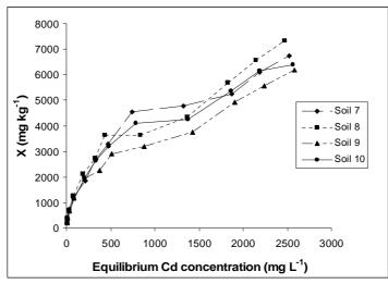
Fig. 2. Relationship between final Cd concentration in equilibrium solution (mgL<sup>-1</sup>) and Cd adsorbed (mg kg<sup>-1</sup>) by acid soils
