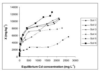
Fig. 1. Relationship between final Cd concentration in equilibrium solution (mg L<sup>-1</sup>) and Cd adsorbed (mg kg<sup>-1</sup>) by calcareous soils
