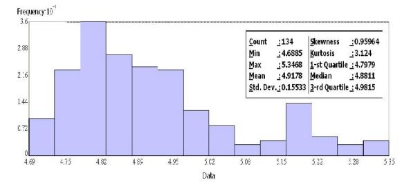
Fig. 3. Diagram of converted hydraulic conductivity frequency
