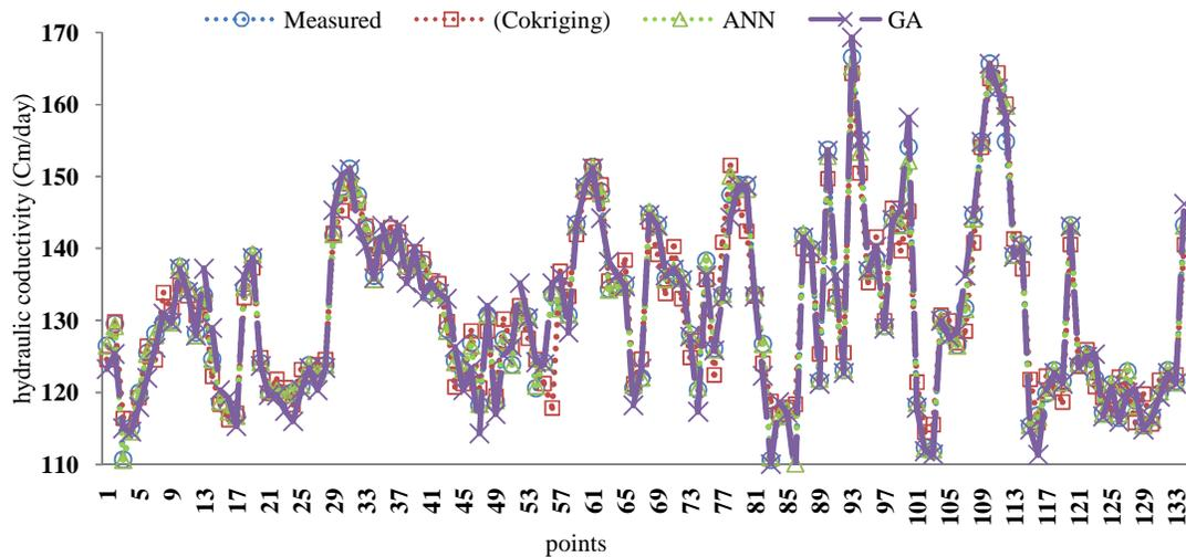
**Fig. 11.** Comparison of predicted values of cokriging and ANN with measured values
