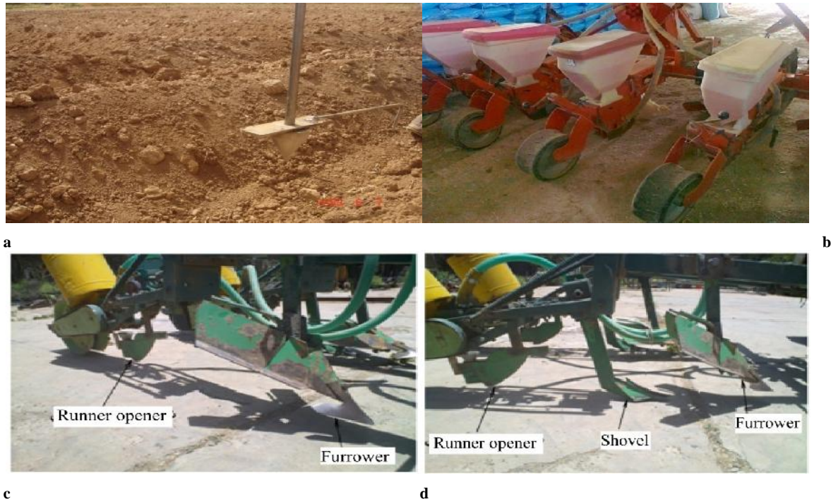
Fig. 1. Different types of planting devices used in the study, a) Hand tool, b) Keveneland planter, c) in-furrow bottom planter, d) in-furrow bottom planter equipped with shovel
