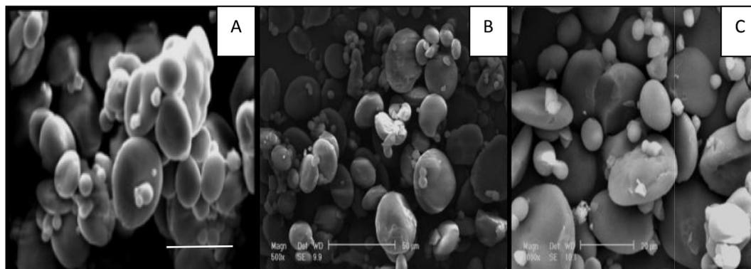
**Fig. 2.** Scanning electron micrographs of the native wheat starch granules (A), heat-moisture treated starch for 14 h (HMT1) (B) and heat-moisture treated starch for 16 h (HMT2) (C). Bars on the micrographs are 20 µm.
