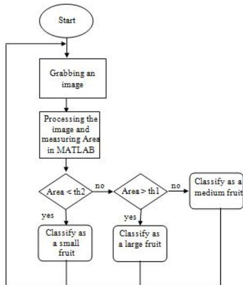
**Fig. 5. Comprehensive sorting algorithm based on area**
