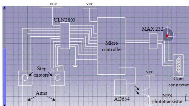
Fig. 3. Layout of the control circuit
