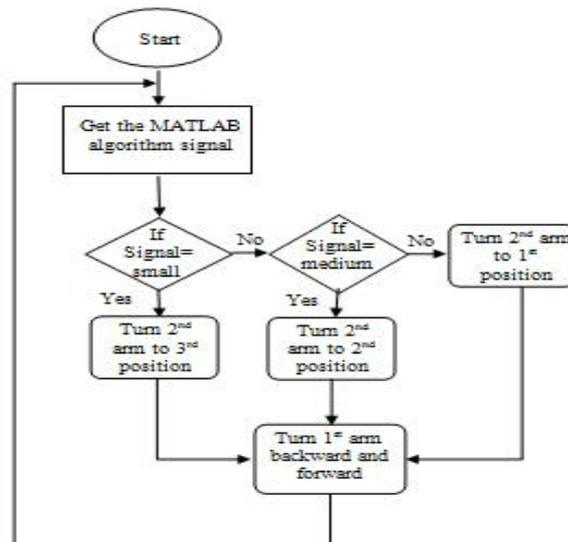
Fig. 7. Algorithm developed for efficient real time image grabbing
