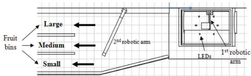
Fig. 2. Top view of the sorting rig
