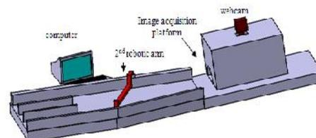
**Fig. 1. Schematic view of the sorting test rig**
