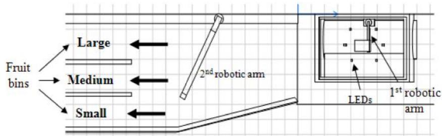
Fig. 2. Top view of the sorting rig
