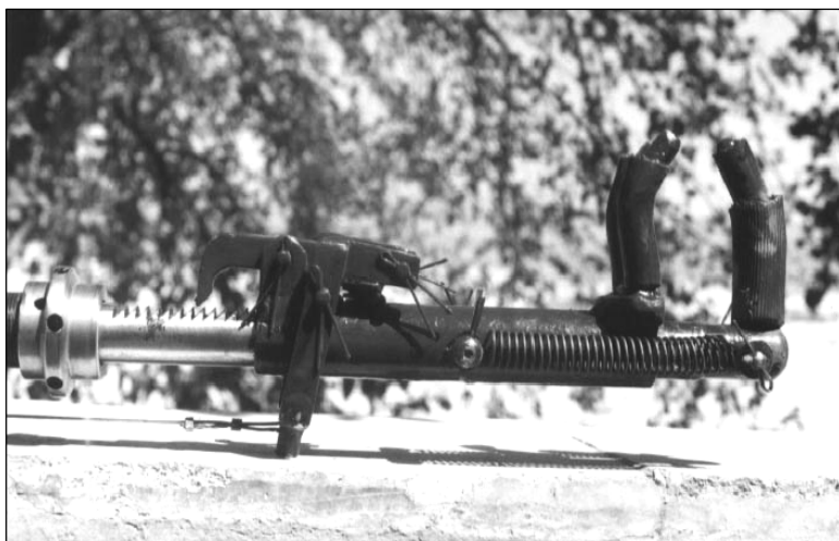
Figure 2. Self-locking gripping fingers of the shaker boom
