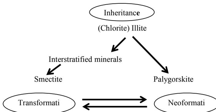
Fig. 6. Pathways for the formation of clay minerals in the studied soils. The thickness of the arrows indicates the importance of the pathway. The parentheses indicate lesser importance.
