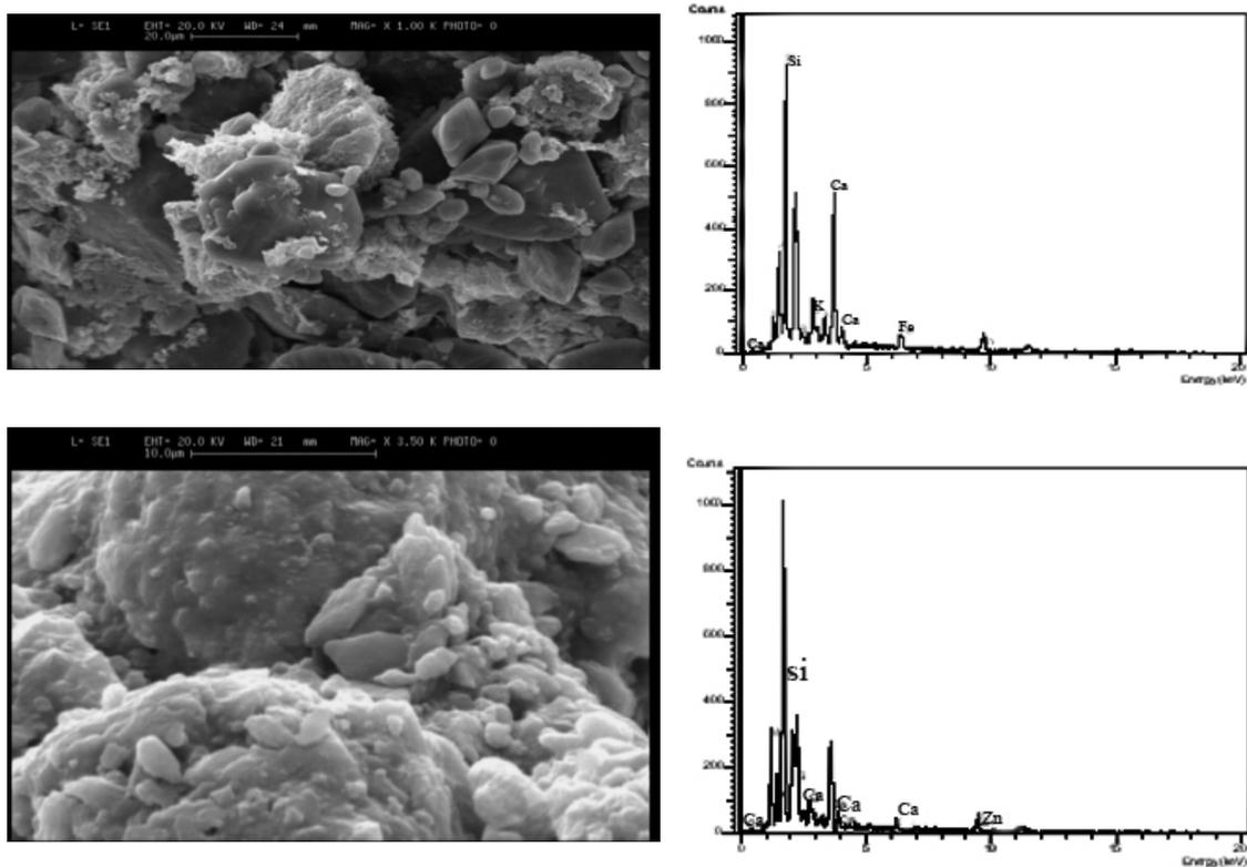
Fig. 5. SEM image of pedogenic carbonates coated with palygorskite (pedon 2, B<sub>k1</sub>) (a) and gypsum (pedon 6, B<sub>v2</sub>) (b) elemental analysis of palygorskite fibres on calcium carbonate nodules and gypsum crystals (SEM-EDX) (c) and (d), respectively
