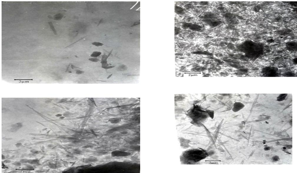
**Fig. 4.** TEM image of the A horizon of pedon 2 ( a), B<sub>tk1</sub> horizon of pedon 3 (b), A<sub>y</sub> horizon of pedon 6 (c) and C<sub>z2</sub> horizon of pedon 7 (d), respectively
