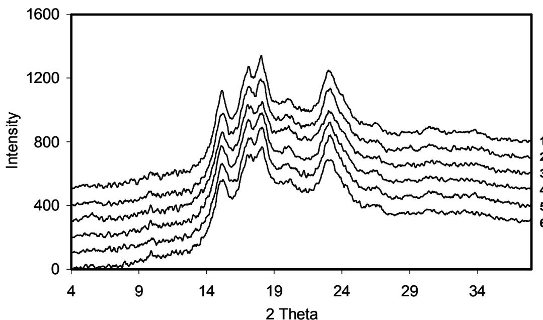
**Fig. 2. X-ray diffraction spectra of the starch component of different rice powders. 1: Tarom Heshmati, 2: Neda, 3: Kamfirouzi, 4: Ramezani, 5: Tarom, 6: Fajr**
